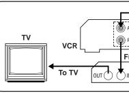
With this connection, you can view one scrambled cable channel while recording another unscrambled channel.
