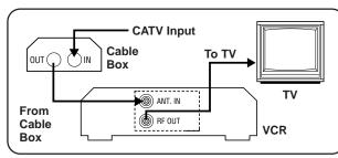
With this connection you can view/record any cable channel including scrambled channels to which you have subscribed.
